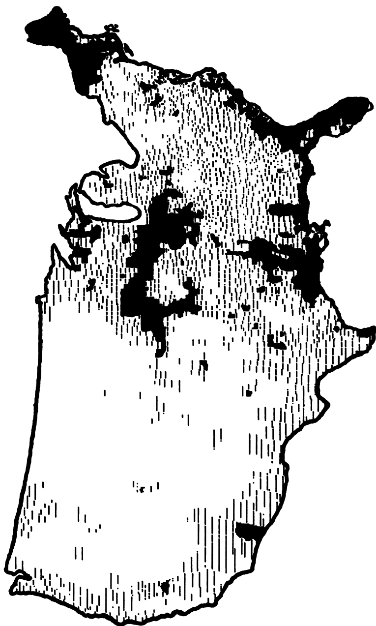
Figure 1. County averaged annual natural sulfur emission rate estimates for all compounds from all sources. Empty = 0.5 to 3, \text{ng S} \cdot \text{m}^{-2} \cdot \text{min}^{-1} ; hatched = 3 to 6, \text{ng S} \cdot \text{m}^{-2} \cdot \text{min}^{-1} ; solid = 6 to 21, \text{ng S} \cdot \text{m}^{-2} \cdot \text{min}^{-1} .
